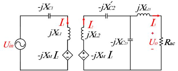
Fig. 5 equivalent circuit of detuned  $S$ - $LCL$  mode.
