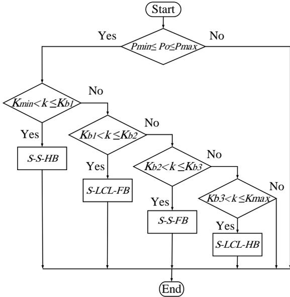
Fig. 8 switching pattern of the proposed detuned IPT.
