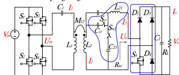
Fig. 1 an IPT system with *S-S/LCL* compensation topology.
