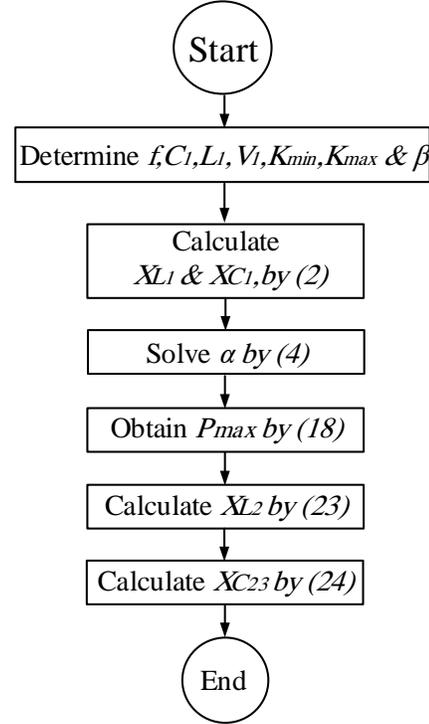
Fig. 7 Flow chart for calculating design parameters.
