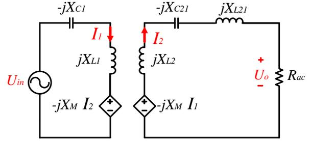
Fig. 2 equivalent circuit of detuned S-S mode.
