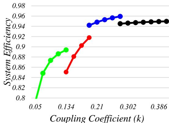
**Fig. 16** Measured efficiencies of the IPT versus misalignment.
