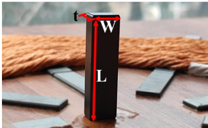
Fig 2. Dimensions of the Type I ferrite core ( L = length, W = width, and t = thickness).
